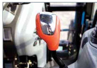
Main gearshift Lever Provides optimal operating capability by smooth gear shifting Hi/Low shift button (Power shuttle only) Convenient Hi/Low shift button does not require clutch and supports F24 x R12 wide range of gear shifting (F40 x R20 with Creeper)
