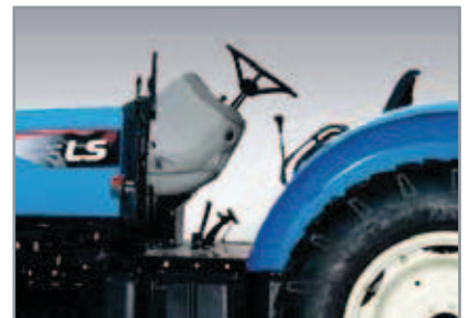
Spacious Flat platform With side mounted gear lever, maximizes space and makes getting on/off tractor easier
