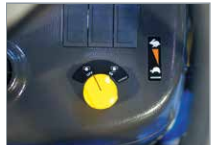
Independent PTO Independent PTO easily operated by switch on the dashboard
