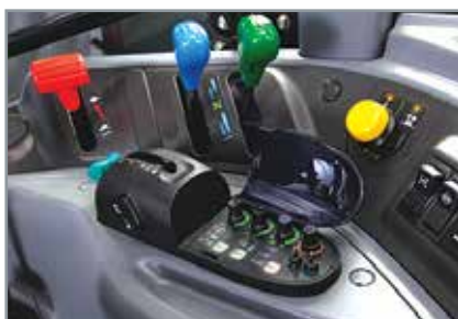
Finger trip type Electro-hydraulic control panel (optional) Integrated switch box with electro-hydraulic control lever puts easy control at your fingertips (More convenient 3 point link control)
